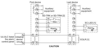
Do not use looped wires under terminals 6 and 10, or 5 and 8 Break wire run to provide supervision of connections
