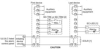
Do not use looped wires under terminals 9 and 7, or 10 and 8. Break wire run to provide supervision of conn
